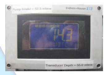
If the well is equipped with a transducer that is great but make sure to know the transducer setting depth and the units the transducer is reporting in (m or feet of water?). Periodically check/calibrate transducer readings with a manual measurement.
